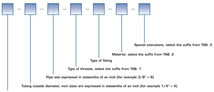
Select M for metric size tubing or P for inch size tubling
